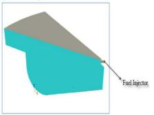
Fig. 1: Sector Geometry of a Direct Injection Natural Gas Engine
