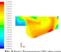
Fig. 5 Static Temperature (30° after ignition)
